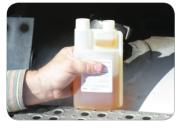
Remove cap from reservoir side of bottle and squeeze desired amount up into reservoir.
