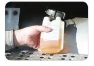
Pour XFT<sup>M</sup> from reservoir into fuel tank sideways to prevent the product from going back down the feeder tube.
